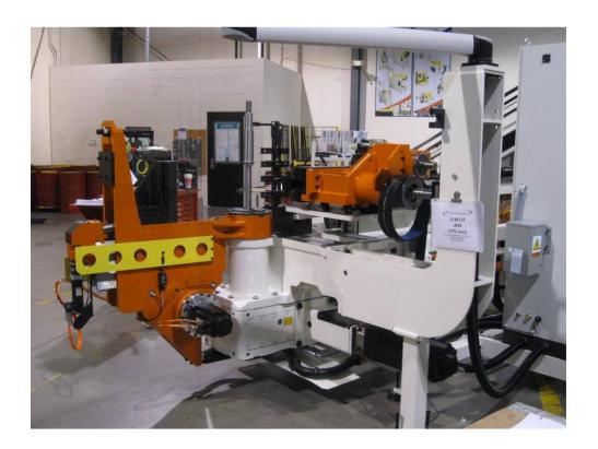
The **AddisonMckee eB80 ESRB** bending machine is an all-electric modular design with bed length variants based upon the same structure – with the capability to design or modify machines specifically to suit individual customer needs. The eB80 ESRB bender has a smaller overall footprint due to the modular design and standard machine mounted guarding.
